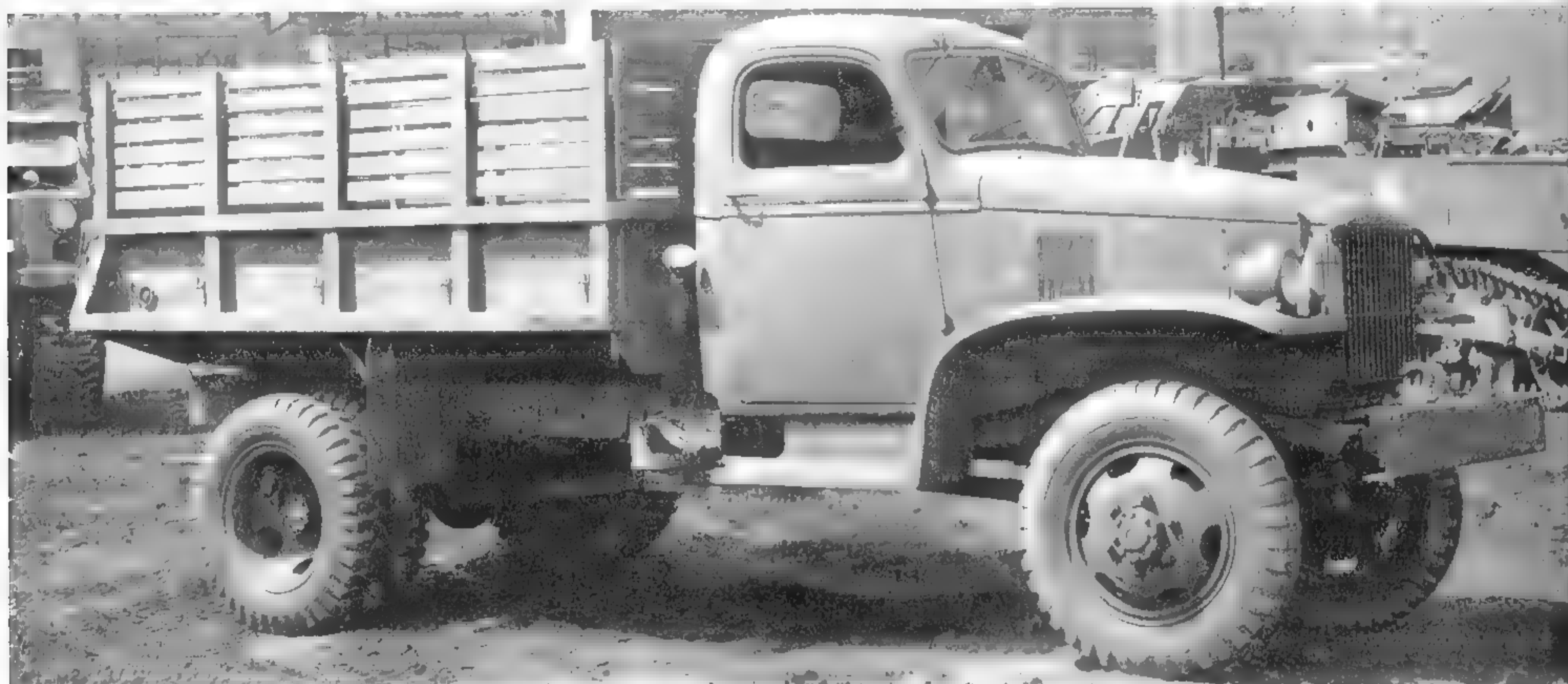
This photograph was taken outside the Army Engineering Standards Vehicle Laboratory in July 1944. It shows a Chevrolet G7107 equipped with a steel cargo bed. The 1 1/2-ton Chevrolet was unusual because it was only built with closed cabs. (U.S. Army photo)
